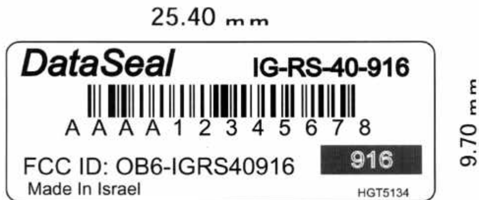
Label placement on the EUT back lateral side
