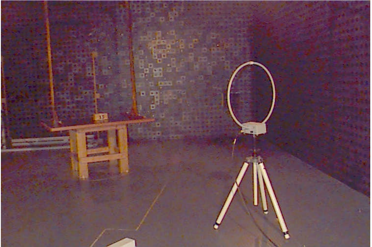
Photograph No.1 Radiated emission measurements test setup with loop antenna, 9 kHz – 30 MHz frequency range, anechoic chamber method
