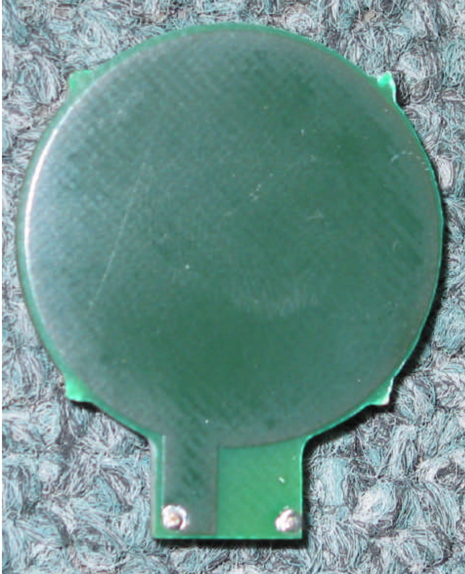
Photograph No.9 Antenna board, printed side
