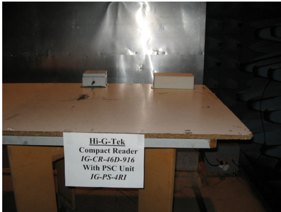
Figure 9. Conducted Emission Test
