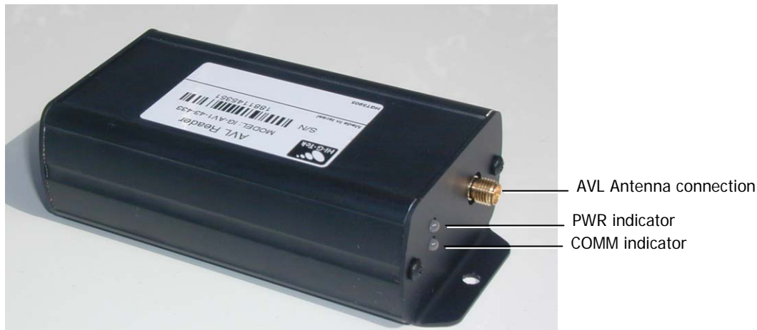
Figure 1-2. AVL Reader Antenna Connection Side
