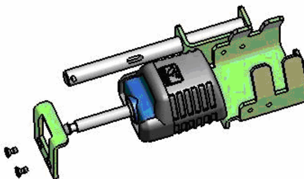
Figure 3-6. Installing the seal inside the housing
