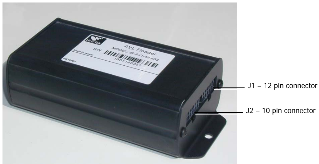
Figure 1-3. AVL Reader Connector Interfaces
