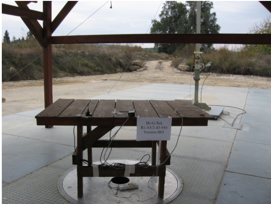
Figure 5. Radiated Emission Test
