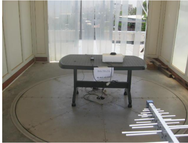
Figure 5. Radiated Emission Test
