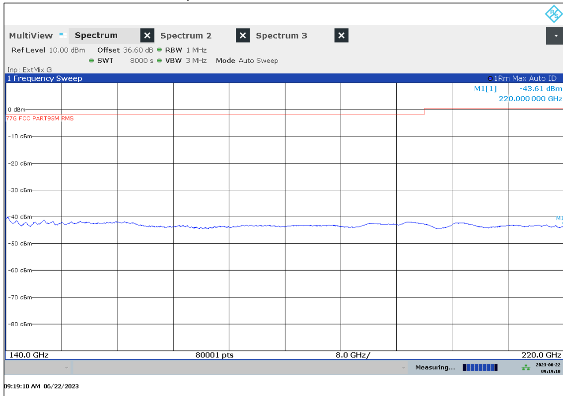
Plot 32: 140 GHz – 220 GHz, valid for specified modes, antenna vertical / horizontal
