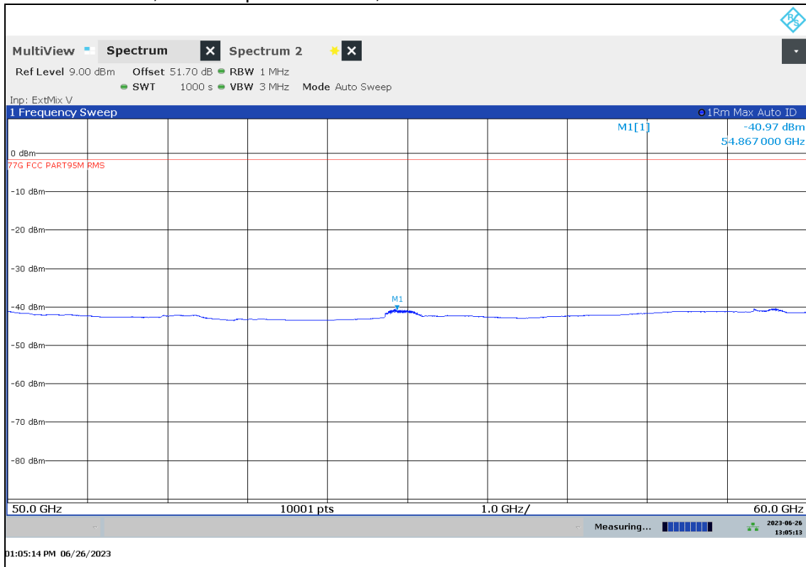
Plot 23: 50 GHz – 60 GHz, valid for specified modes, antenna vertical / horizontal
