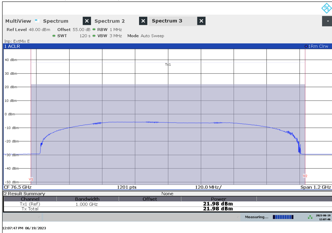
Plot 8: EIRP Mean Power (Channel Power), Mode 03, RMS detector, T_{nom} / V_{nom}
