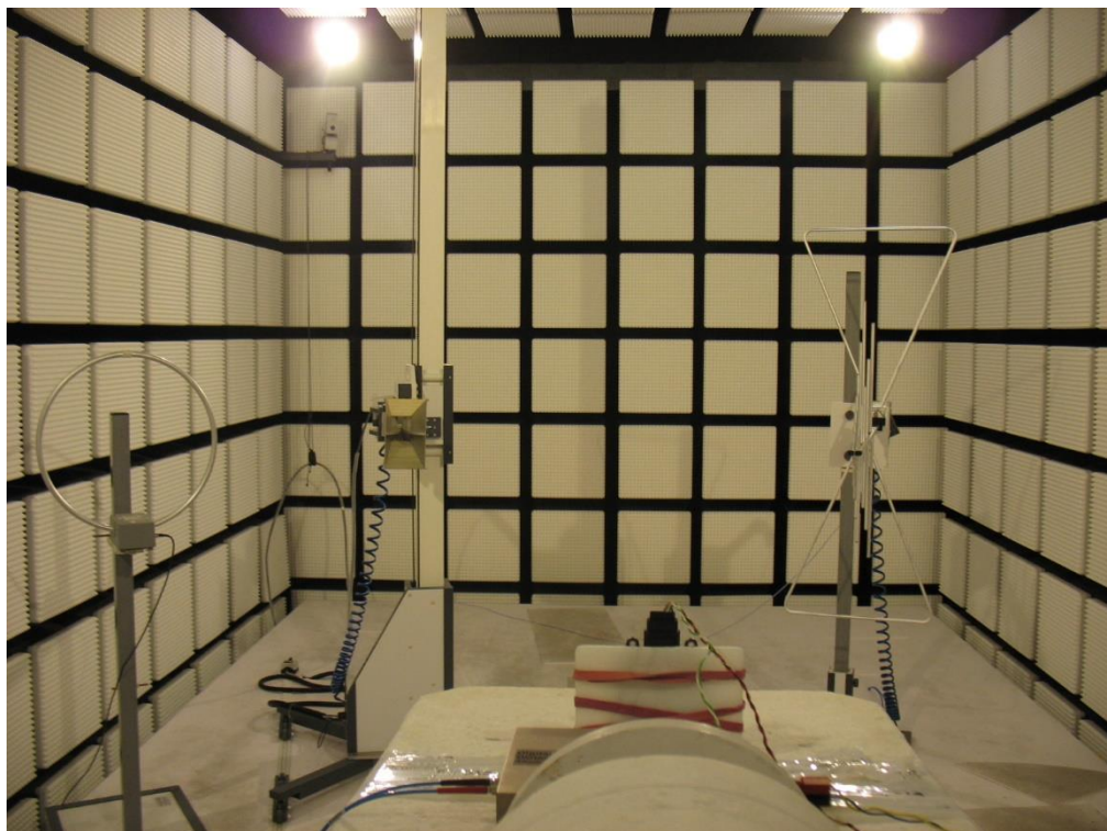
Photo 6: RSE set-up 1 GHz to 18 GHz, low / mid / high frequency
