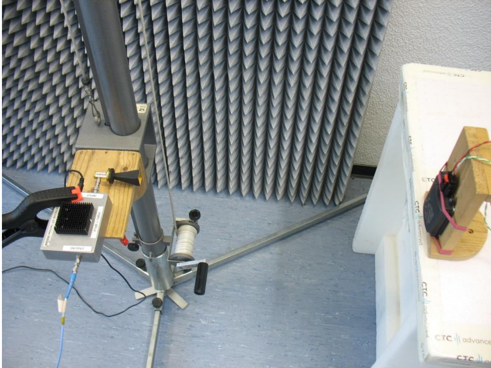
Photo 7: RSE set-up 18 GHz to 110 GHz, low / mid / high frequency
