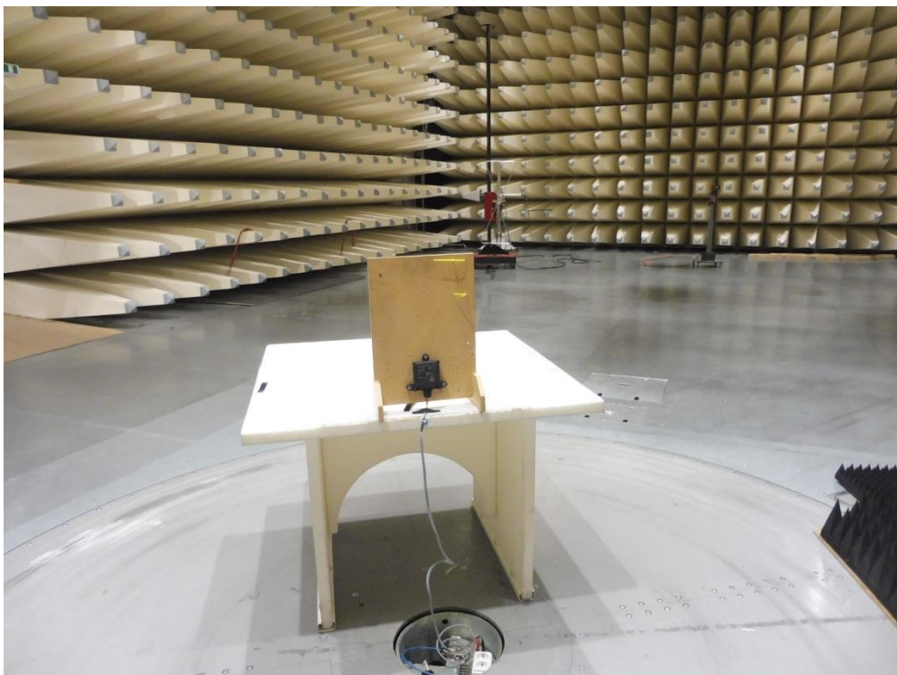
Photo 2: RSE set-up 30 MHz to 1 GHz, low / mid / high frequency
