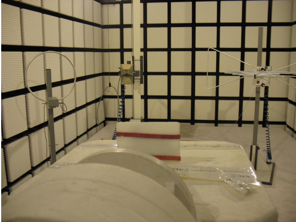
Photo 3: RSE set-up 1 GHz to 18 GHz, low / mid / high frequency
