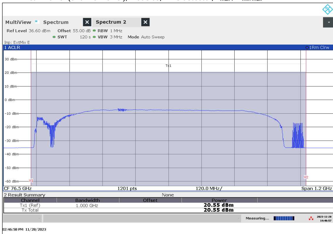
Plot 51: EIRP Mean Power (Channel Power), Mode 63, RMS detector, T_{max} / V_{min-max}
