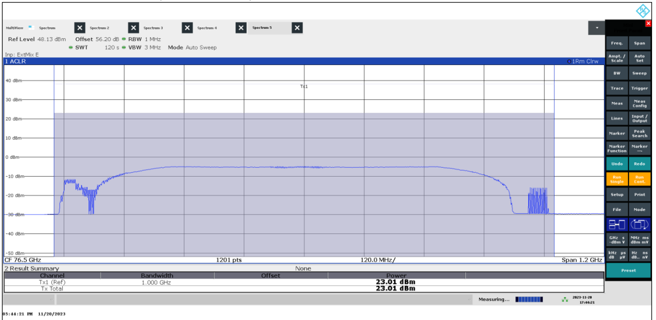
Plot 49: EIRP Mean Power (Channel Power), Mode 63, RMS detector, T_{nom} / V_{min-max}
