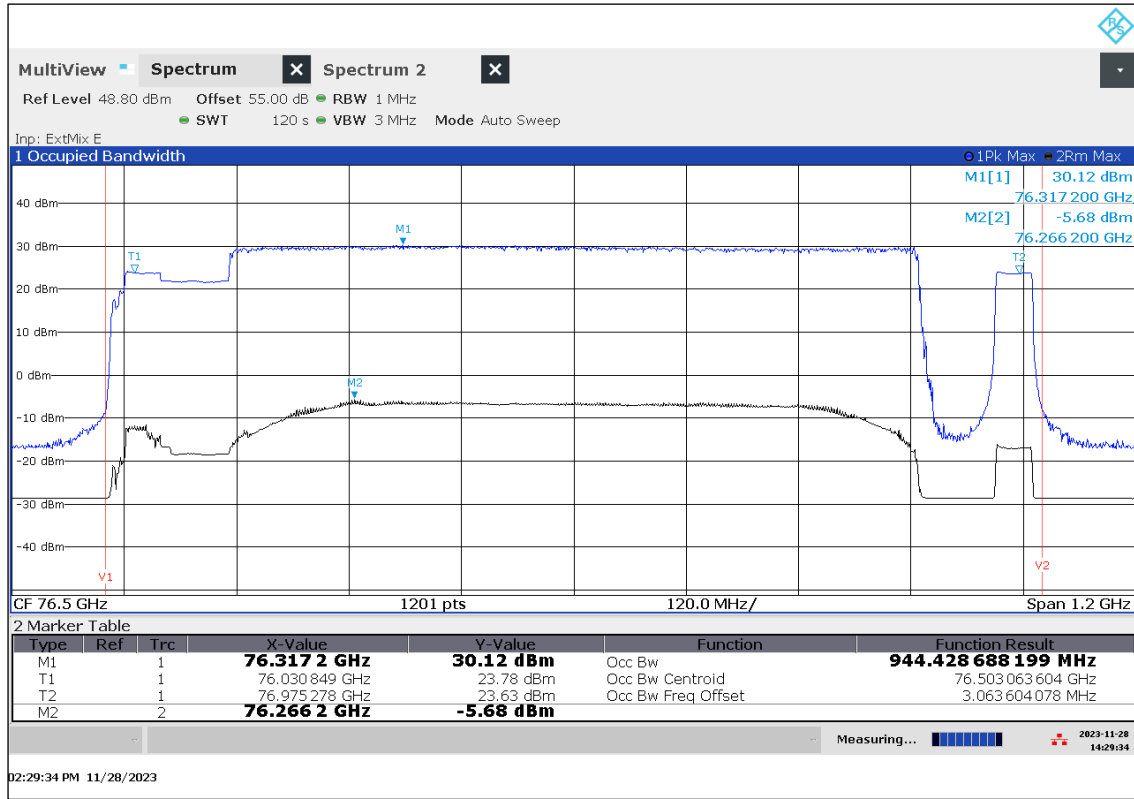
Plot 21: OBW, Mode 51, T_{max} / V_{min-max}
