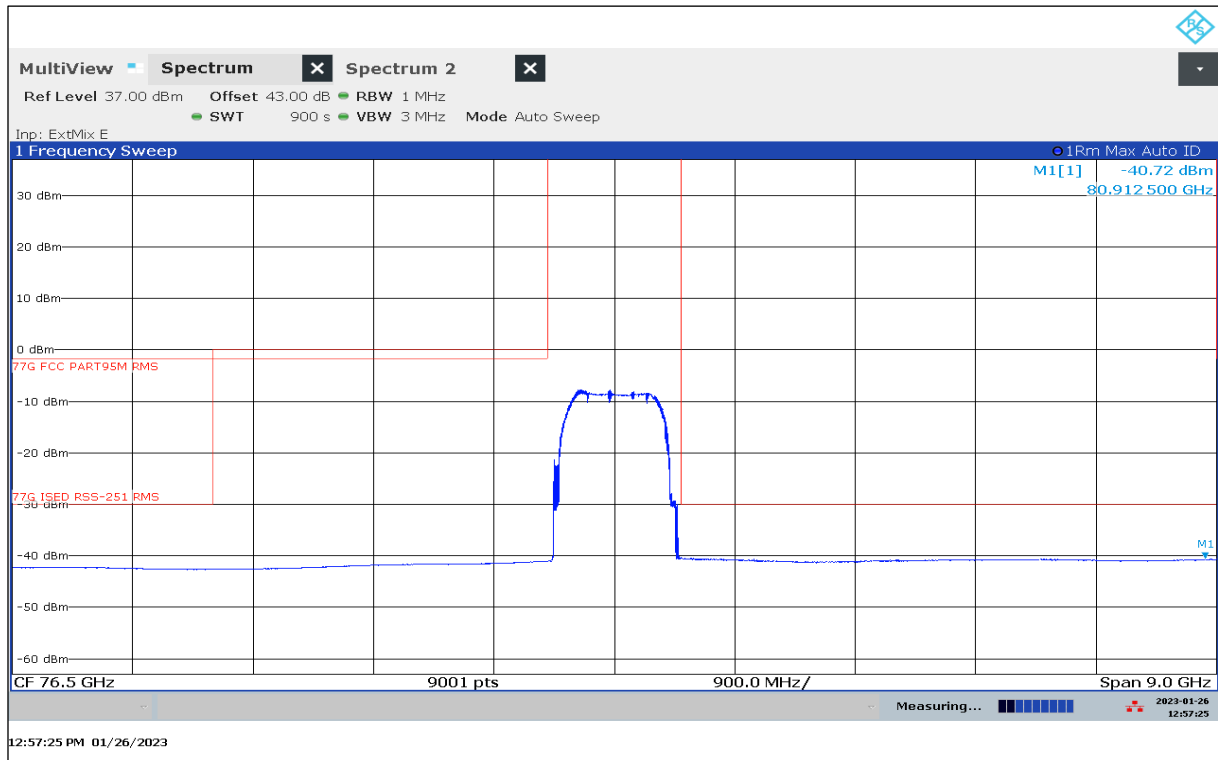
Plot 71: 72 GHz – 81 GHz, Mode 63, antenna vertical / horizontal
