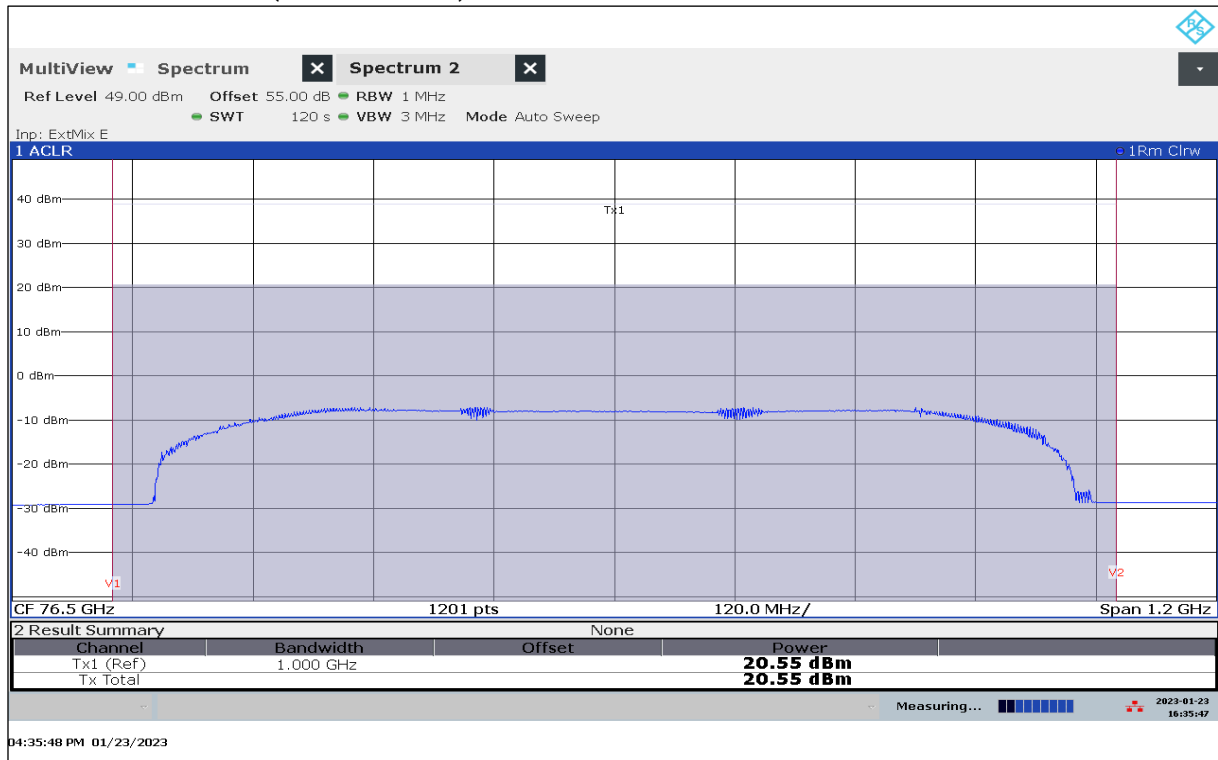
Plot 43: EIRP Mean Power (Channel Power), Mode 39, RMS detector, T_{nom} / V_{min-max}
