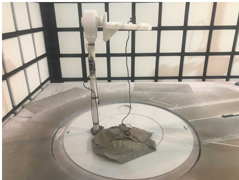
Photo 2 1-18 GHz test setup
