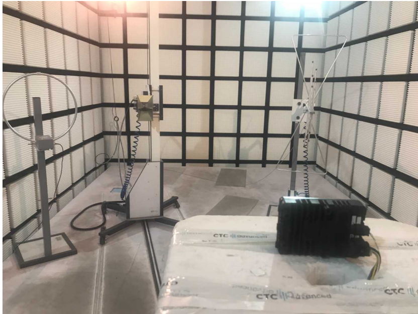
Photo 3 1-18 GHz test setup
