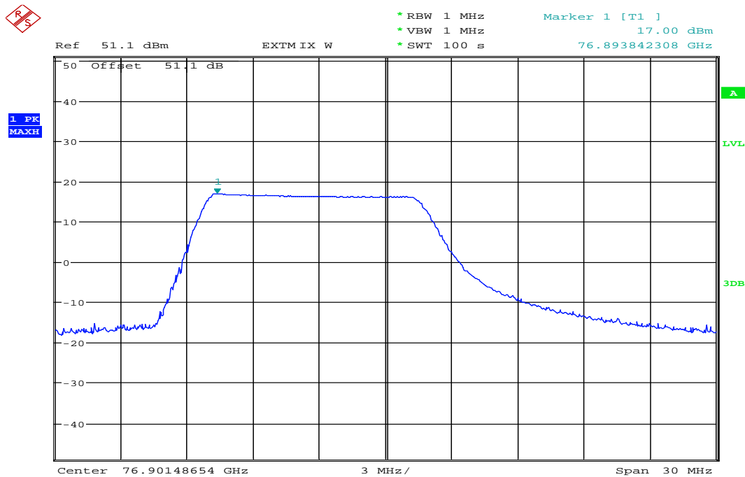
Plot 41: EIRP (Peak detector), T_{min} / V_{min} - V_{max} , upper frequency, low power
