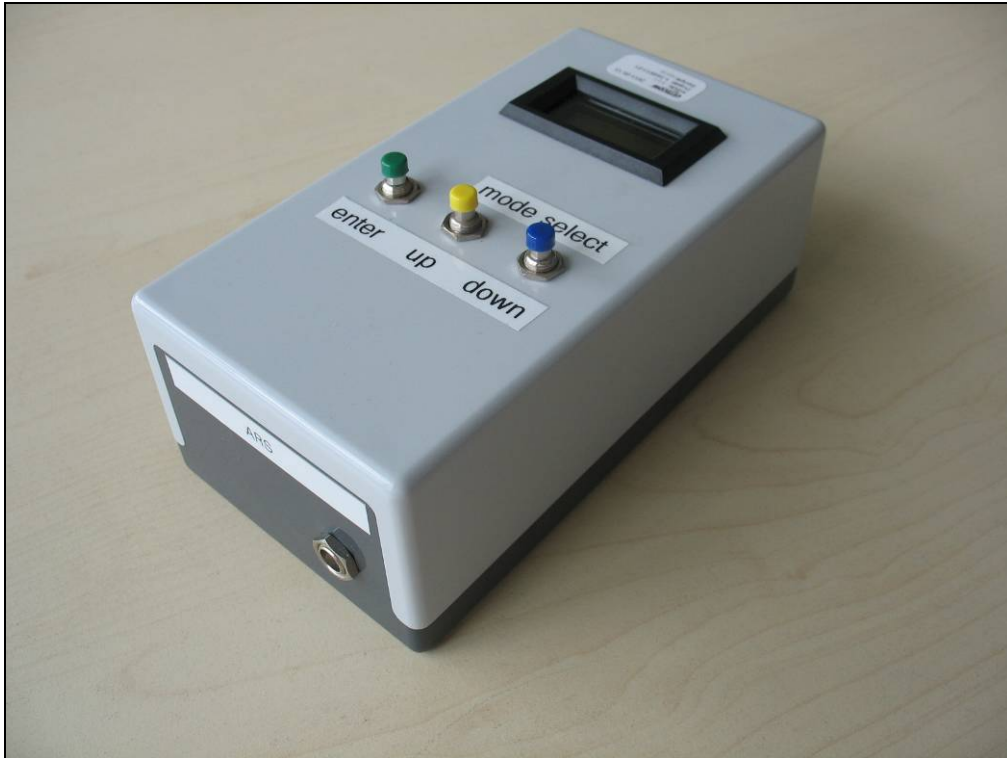
Photo 16: Mode switch box
