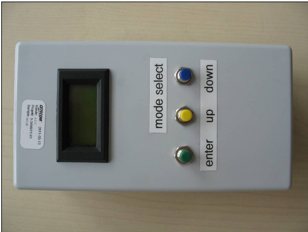
Photo 13: Mode switch box
