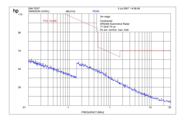
Settings: RBW/VBW : 200 Hz up to 150 kHz, 9 kHz up to 30 MHz,
