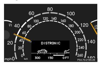
With the electronic key in starter switch position 2, the distance warning lamp in the speedometer dial comes on and goes out with the engine running.
