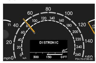
When Distronic system is activated, one or two segments around the speed stored in memory light up in the speedometer dial.
