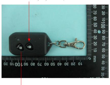
2. Push transmitter BTN2(unlock) one time, door unlock
