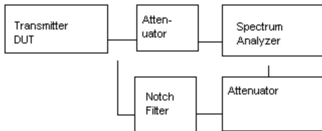
Method of Measuring Conducted Spurious Emissions
