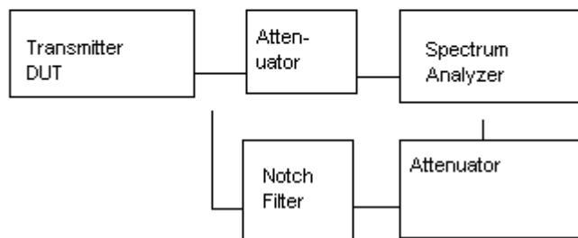
Method of Measuring Conducted Spurious Emissions
