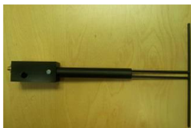
Figure 1 – MVG COMOSAR Validation Dipole
