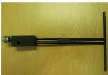
Figure 1 – MVG COMOSAR Validation Dipole
