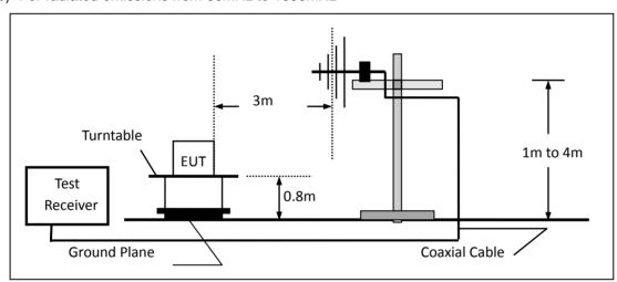
(c) For radiated emissions above 1000MHz
