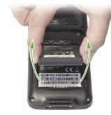
Place the replacement battery in its slot.
