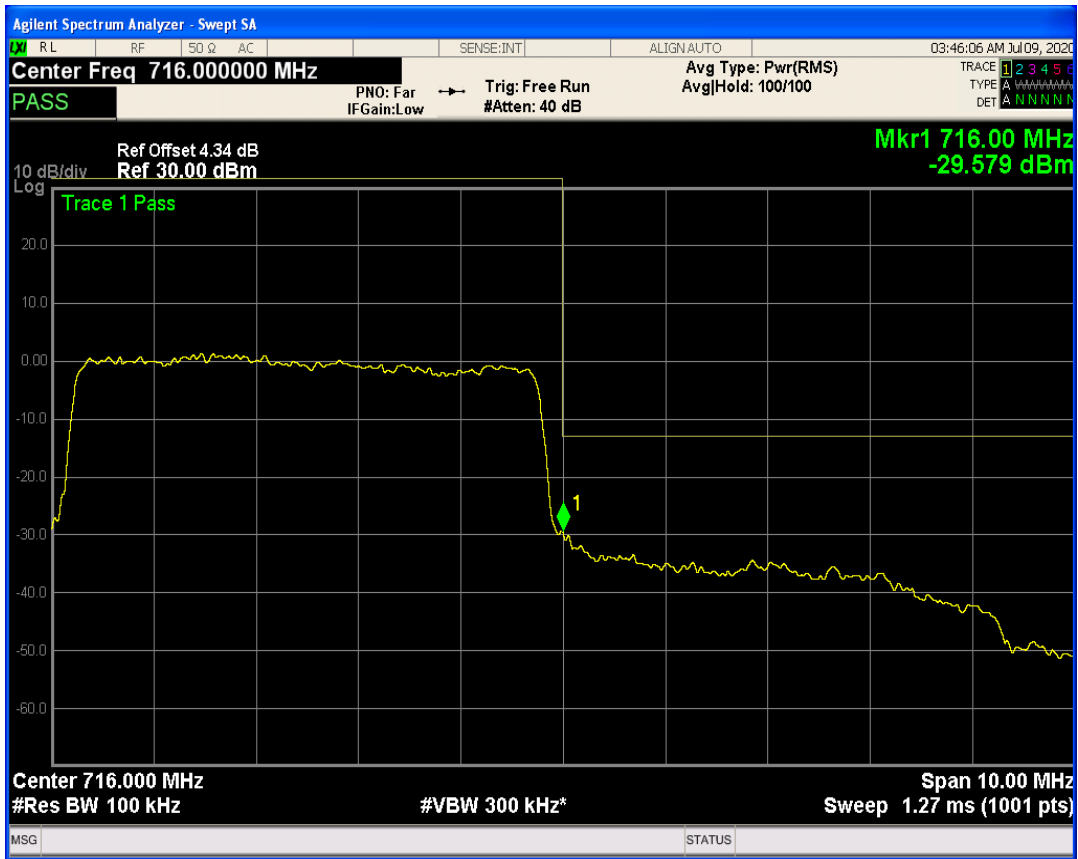
LTE Band12 QAM16 BW=5MHz Channel=23155 RB Size=1 Position=#0
