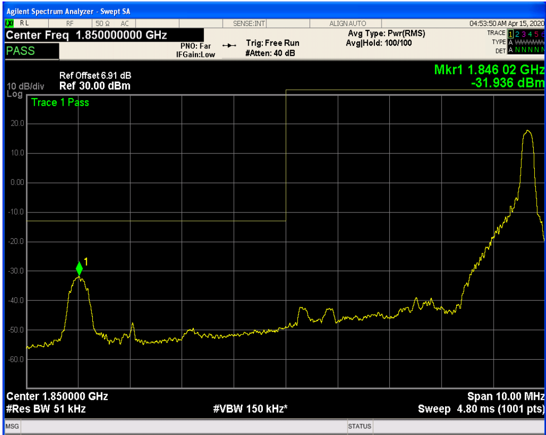
LTE Band2 QAM16 BW=5MHz Channel=18625 RB Size=1 Position=#Max
