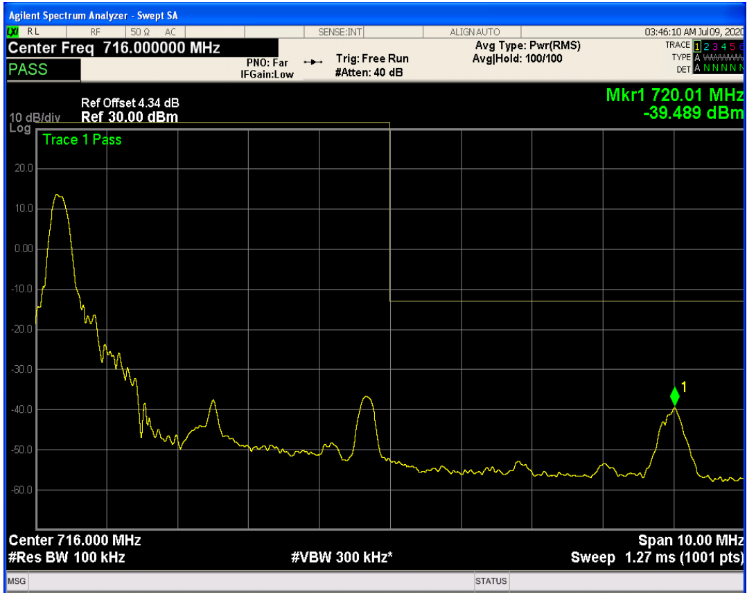
LTE Band12 QAM16 BW=5MHz Channel=23155 RB Size=1 Position=#0
