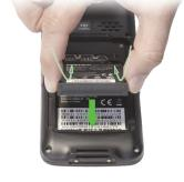
Assemble the cover as shown in the figure and fix it with the two screws previously removed.
