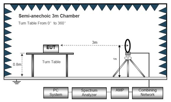
(B) Radiated Emission Test-Up Frequency 30MHz~1GHz
