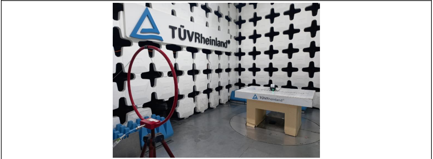
Photo n°1 – Radiated emission 9KHz – 30MHz
