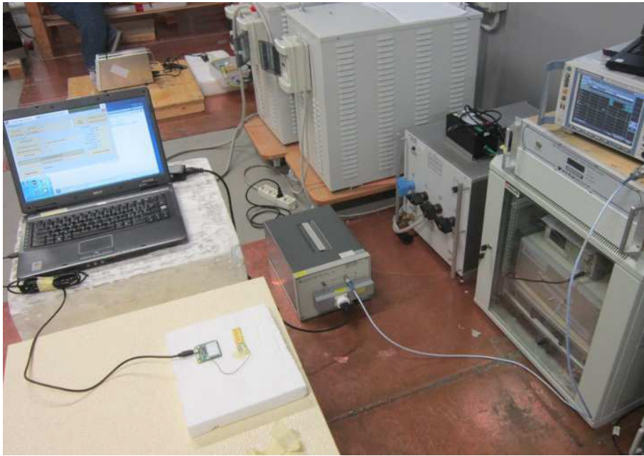
AC Power Conducted Emission
