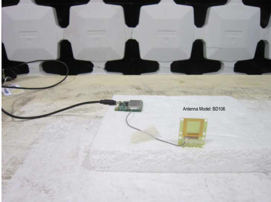
Radiated Emission Above 1GHz
