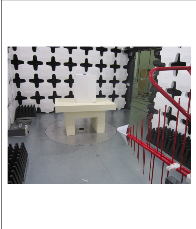
RADIATED TEST SETUP
