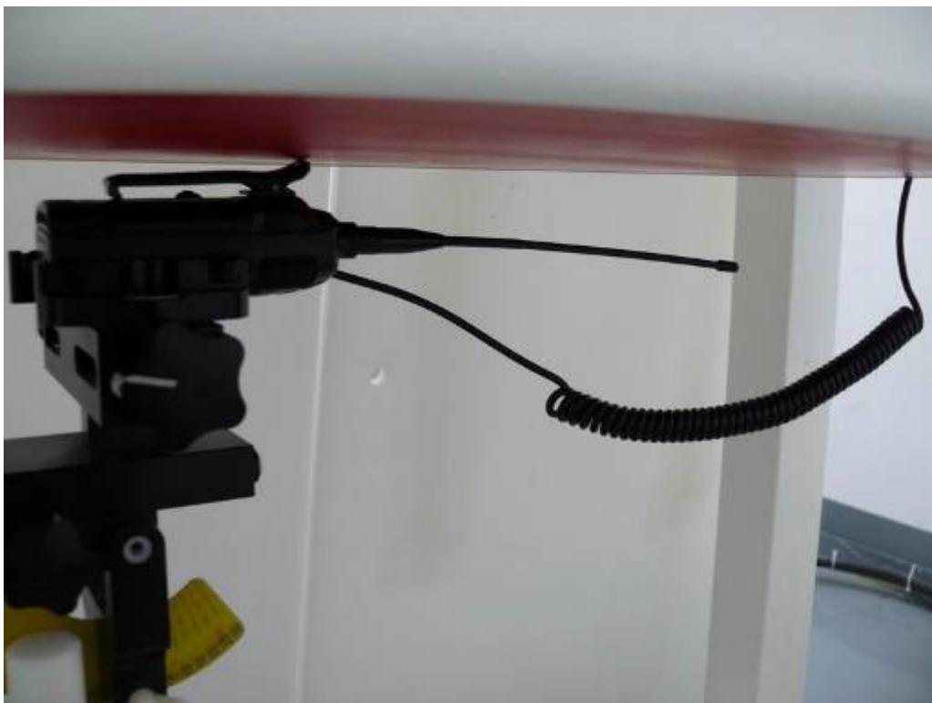
Picture 6: Body-worn with Microphone, The EUT display towards ground, Belt clip attach the Phantom
