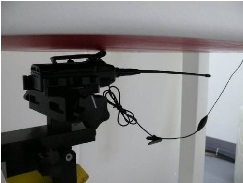
Picture 5: Body-worn with Earphone, The EUT display towards ground, Belt clip attach the Phantom
