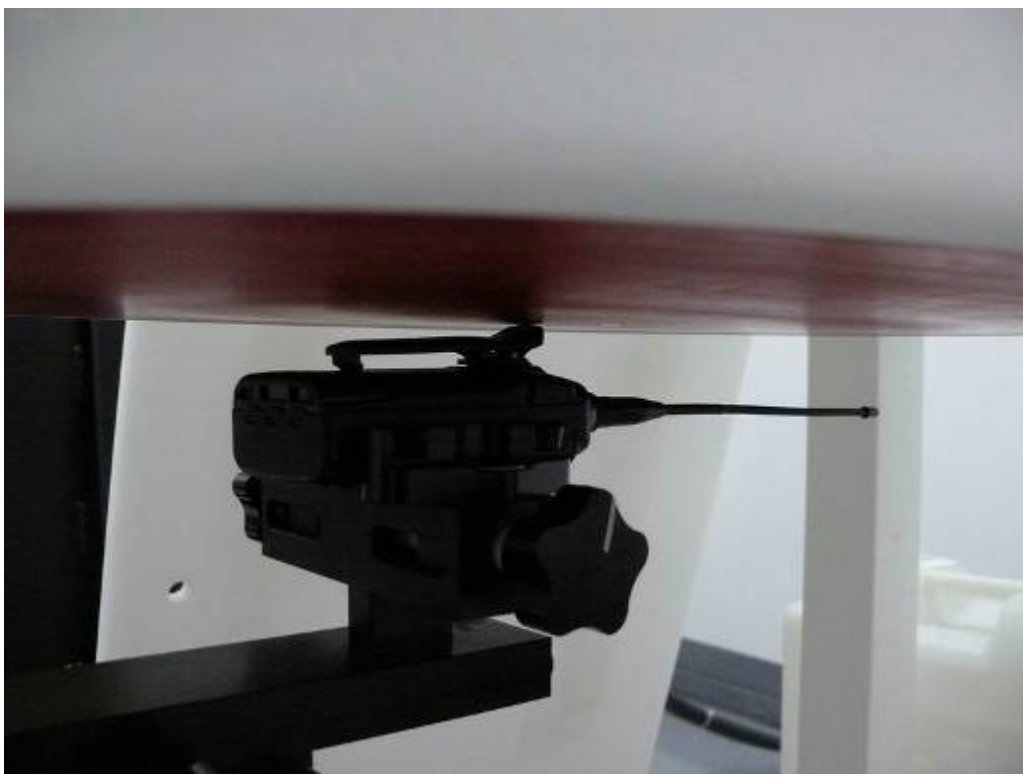
Picture 4: Body-worn, The EUT display towards ground, Belt clip attach the Phantom
