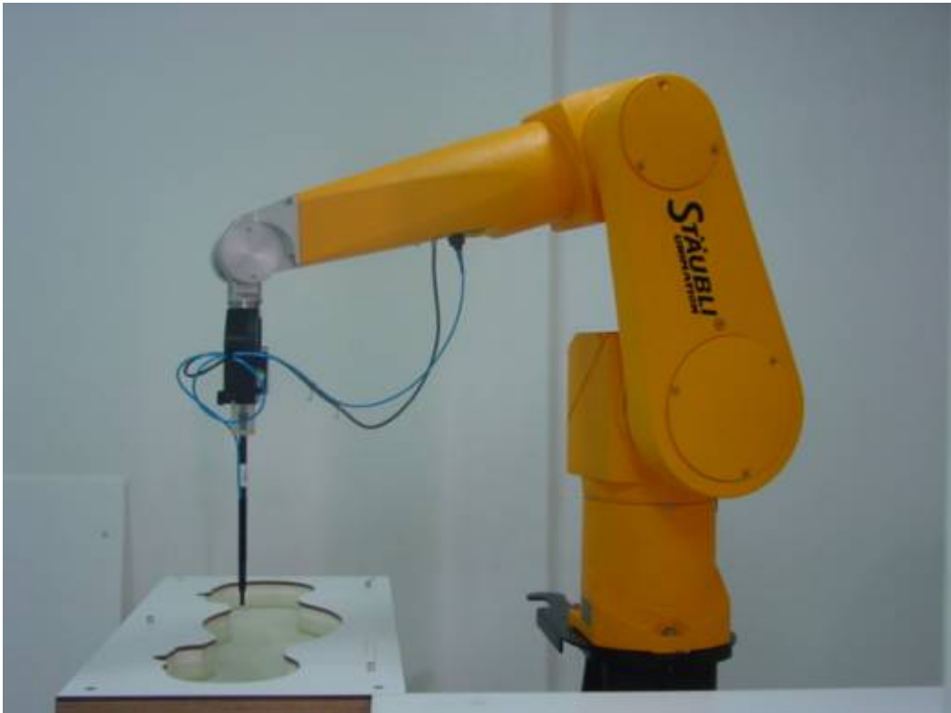
Picture 1: Specific Absorption Rate Test Layout
