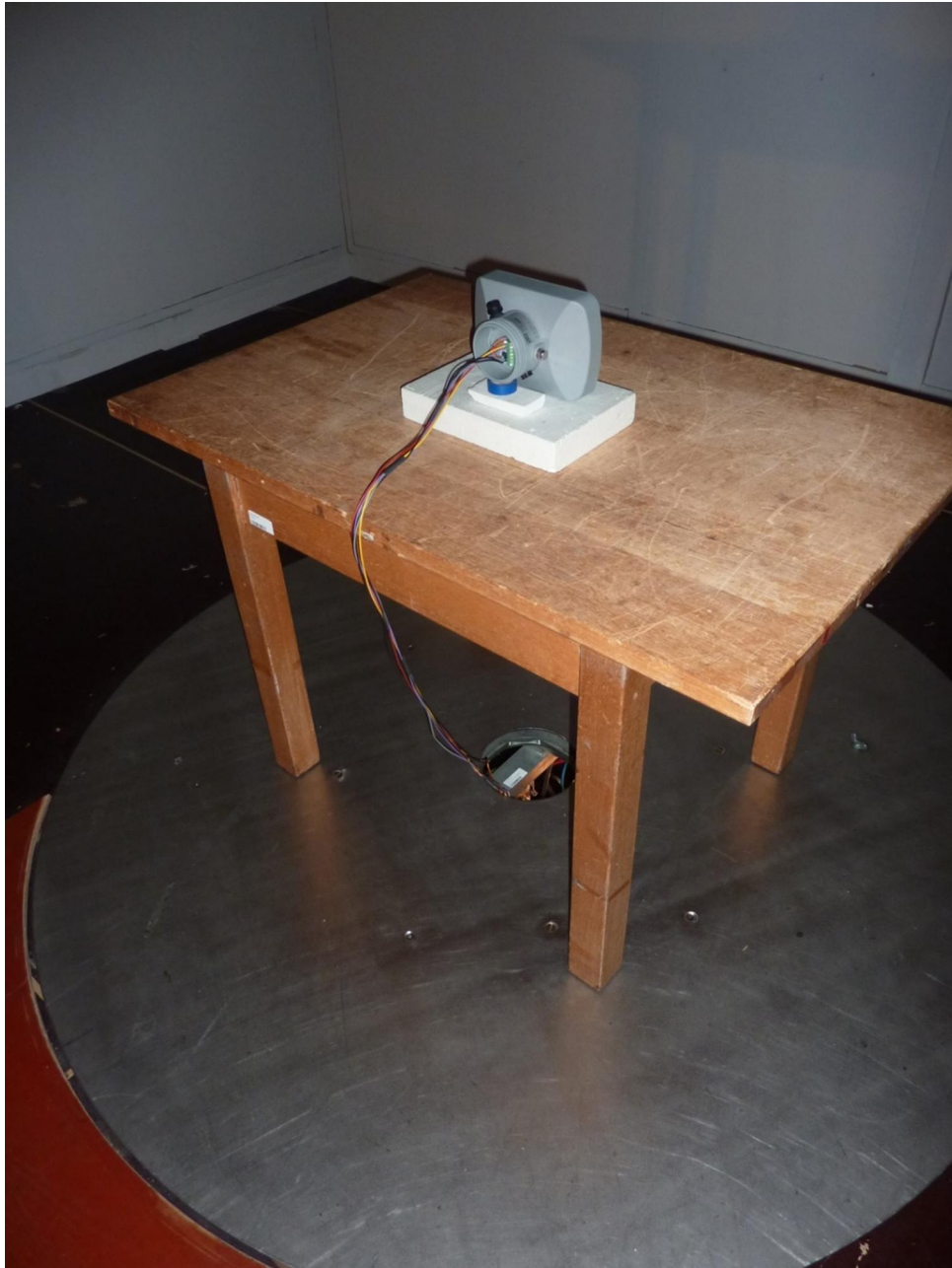
172171_9.JPG: RLS, test setup open area test site (pos. 2)
