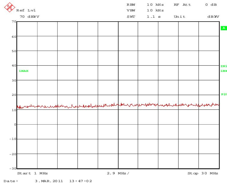
No significant emissions found, above the noise floor of the measuring system, so no measurements on the outdoor test site were carried out.
