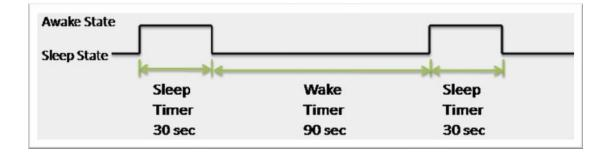
The above diagram shows the transitions between the Sleep state and Awake state based on the sleep and wake timers.
