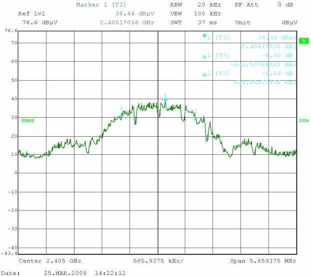
Channel 11 (2405 MHz) 6 dB Bandwidth: 1.573 MHz
