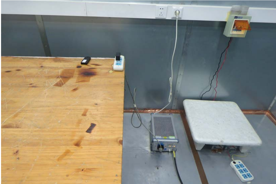
Picture 2: Conducted Emissions Test Setup
