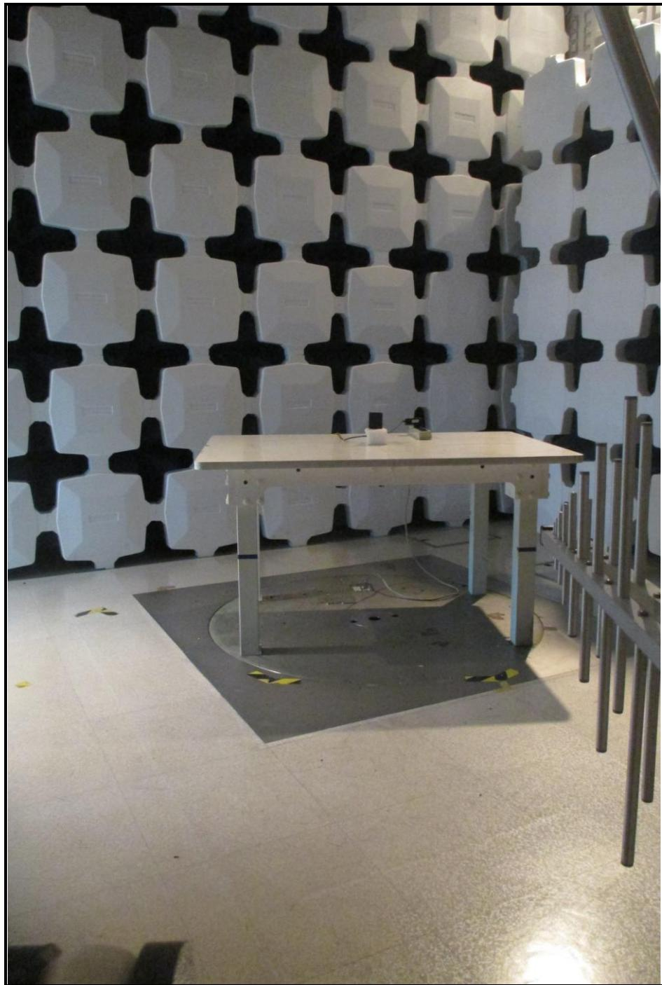
RADIATED EMISSION TEST ABOVE 1GHz
