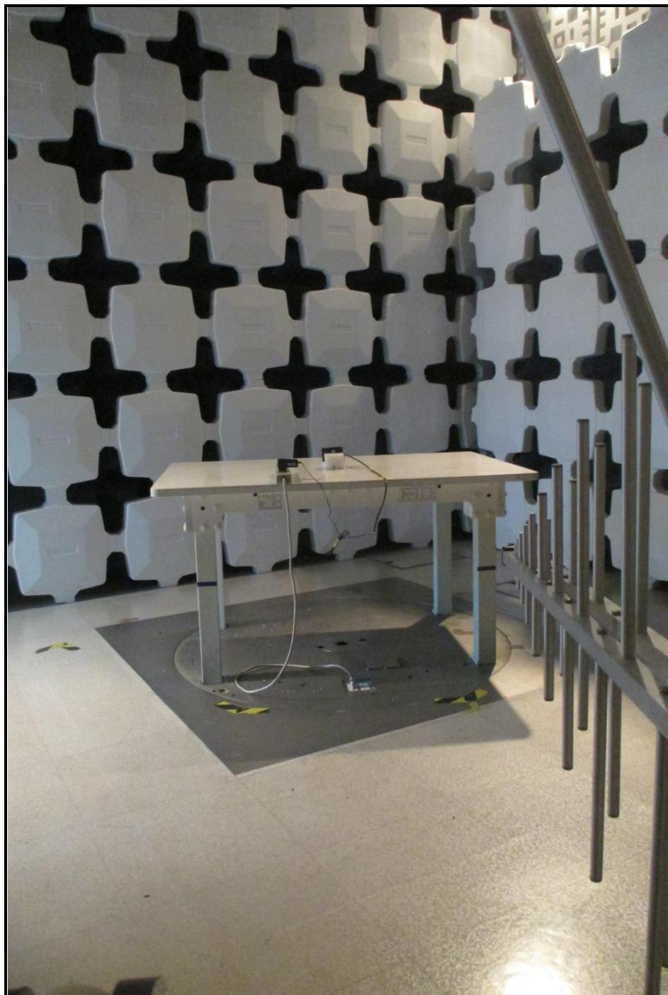
RADIATED EMISSION TEST BELOW 1GHz
