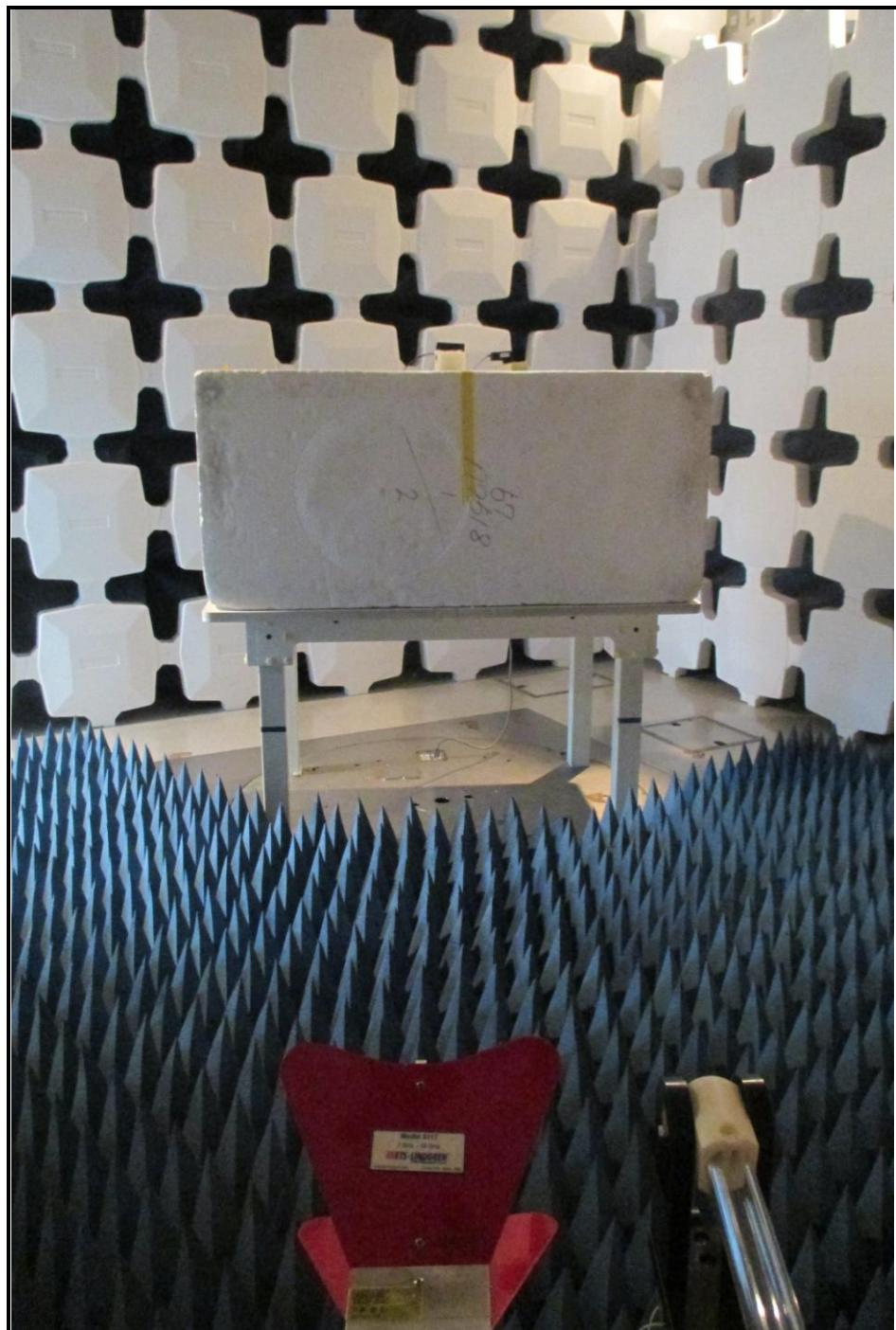
RADIATED EMISSION TEST ABOVE 1GHz
