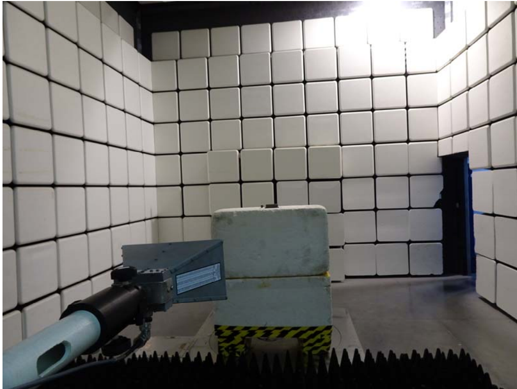
Picture 1: Radiated Spurious Emissions Test setup
