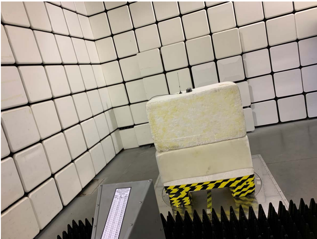
Picture 1: Radiated Spurious Emissions Test setup
