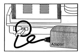
1. Plug the exclusive power supply to POWER connector on the GVP.
