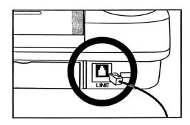
3. Plug a phone cable into the jack labeled LINE on the back of the GVP.
