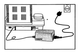
2. Connect the power cable to the power adapter and plug the other end of the cable into a wall outlet.
