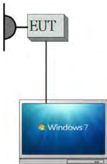
Fig. 2-1 Radiated Emission & Conducted (Antenna Port) Configuratio
