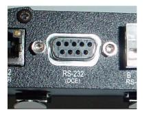
Hardware handshaking using the CTS/RTS lines is provided. The CTS/RTS lines can be configured to reflect the status of the local unit's input buffer. The 455U supports XON/XOFF flow control.
