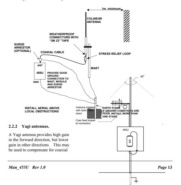
cable loss for installations with marginal radio path.
