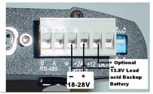
The 12-15 V Supply may be used to charge a backup battery (12V Lead-acid) when the main supply is available, and the module will automatically change over to run from the backup battery in the case of main supply failure.
