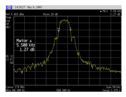
The declared bandwidth has been confirmed even though it is slightly higher that the calculated and measured necessary bandwidth and therefore allows for measurement uncertainties.
