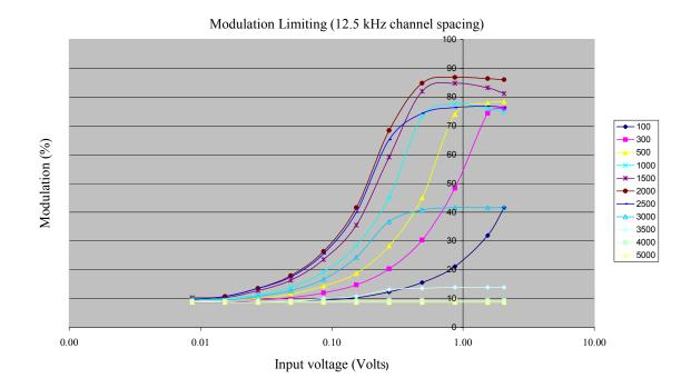
A curve or equivalent data that shows that the equipment will meet the modulation requirements of the rules under which the equipment is to be licensed.
