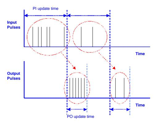
As well as accumulating the pulse input, the 905 module will also calculate the rate of pulses. Pulse rates are treated as an "internal" analogue input and are configured with analogue sensitivities for change-of-state transmissions. The maximum pulse rate corresponding to 20mA output may be configured by the user.
