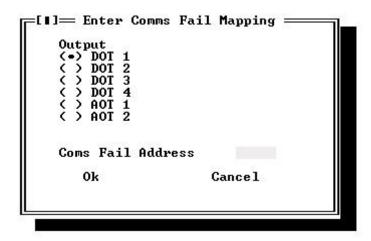
Enter the output at which the comms fail indication is to appear, and the address for which the comms fail should be indicated.
