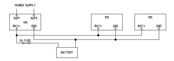
The internal power supply of the 905 module can supply a maximum 12V load of 700mA. In order to achieve this, the input power supply must be above 15VAC or 17VDC. Using these figures, it can be determined whether there is enough supply for more than one module - allow 100mA for recharging a battery.
