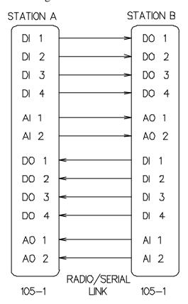
In this configuration, the "PO" Pulse output is inactive and no special action is taken on "Comms fail", "Mains fail" or "Battery Low". "DI 1" is configured as a digital and not a pulse input.
