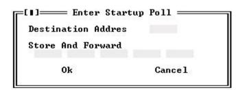
Enter the address of the unit to poll in the "Destination address" section, and the addresses of any intermediate units required to reach this unit in the "Store and Forward" section (starting with the nearest repeater address).
