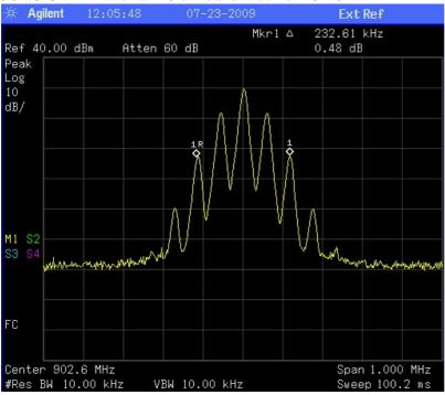
915 MHz with a -20 dB bandwidth of 230 kHz
