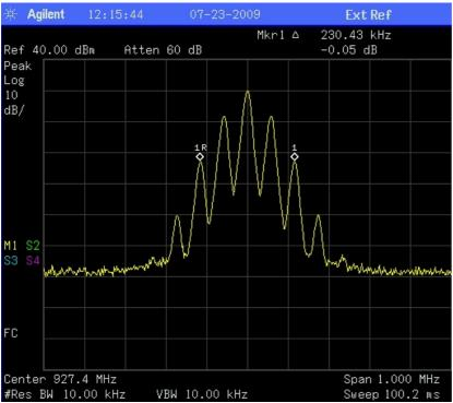
When operating with 100 channels, in any 20 second period the transmitter was observed to transmit twice transmitting every 10 seconds.
