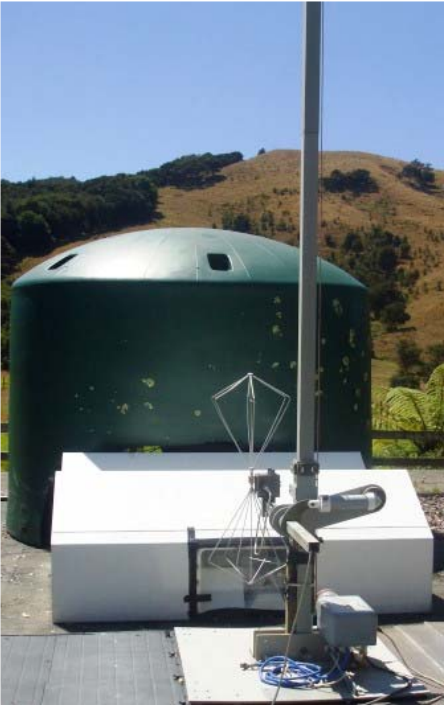
Schwarzbeck Biconnical Antenna (30 – 300 MHz)
