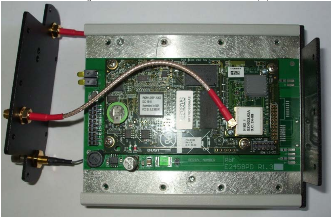
Rear cover removed showing the main rear board with the Wi Hart Module boards (x2) attached
