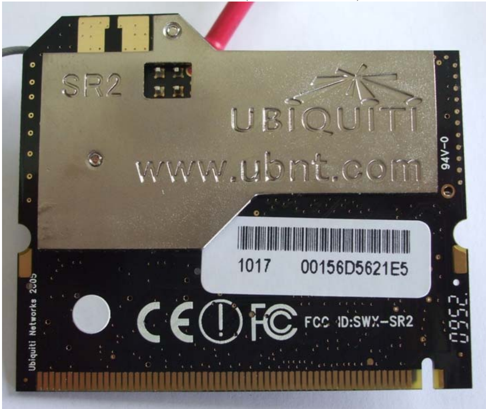
Rear view of the Wi Fi radio module board (FCC ID: SWX-SR2)
