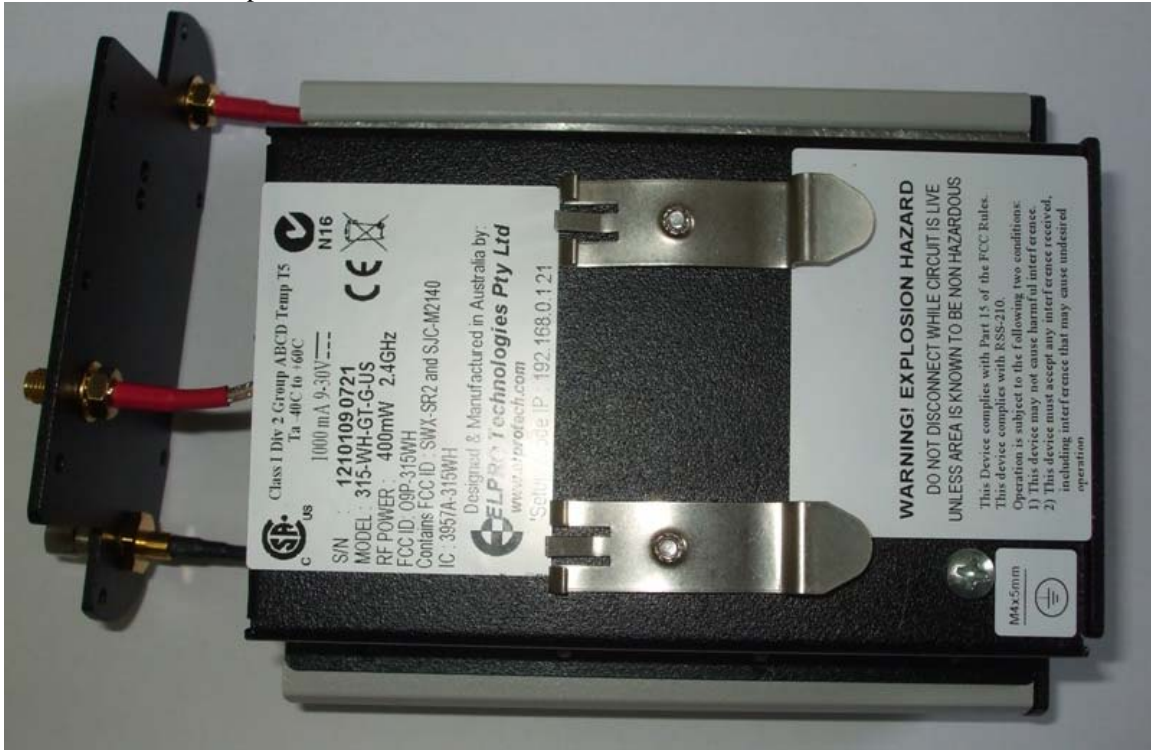
Rear cover with end top antenna cover removed
