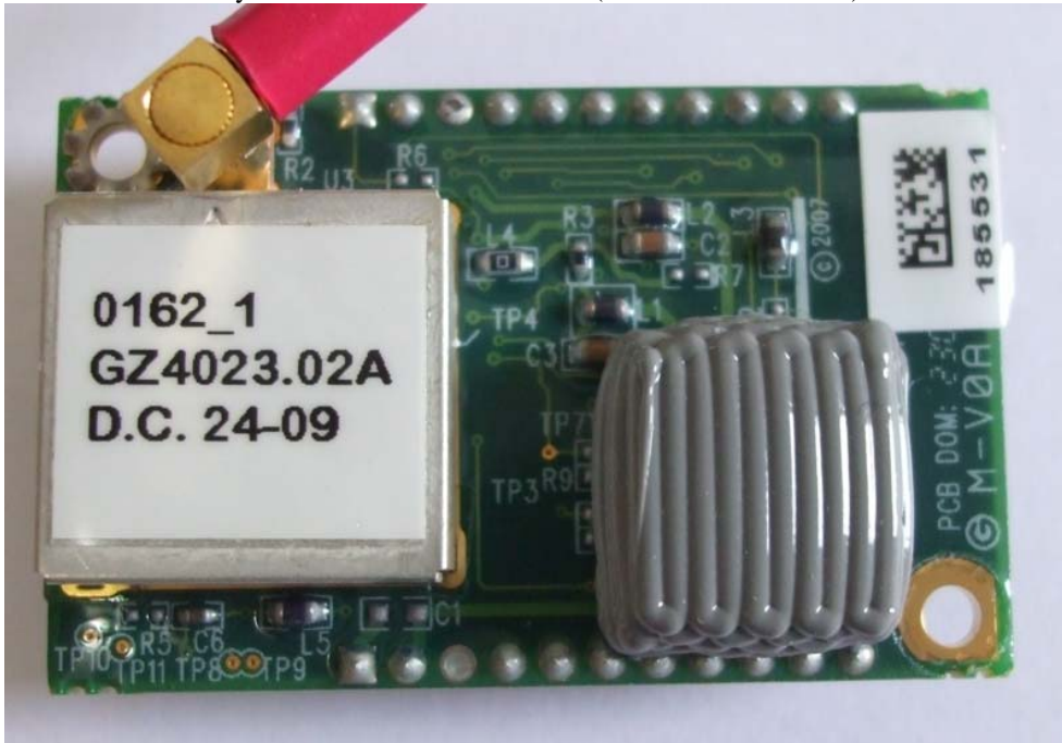
Rear of the ancillary Wi Hart radio module board (FCC ID: SJC-M2140).
