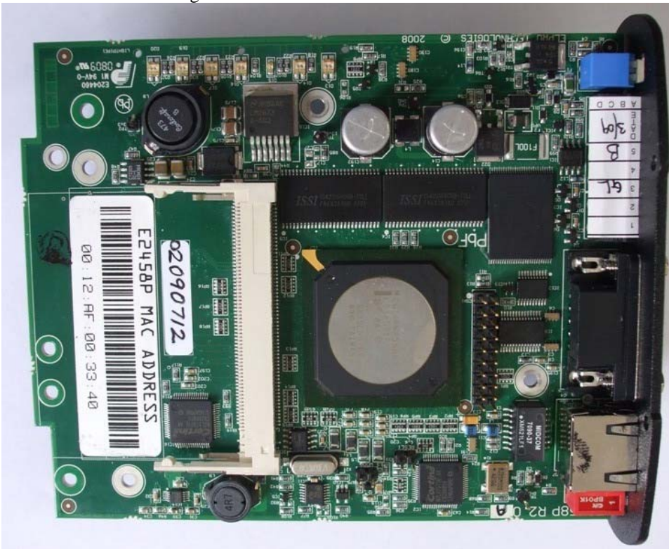
Front main board showing the Wi Fi module board removed
