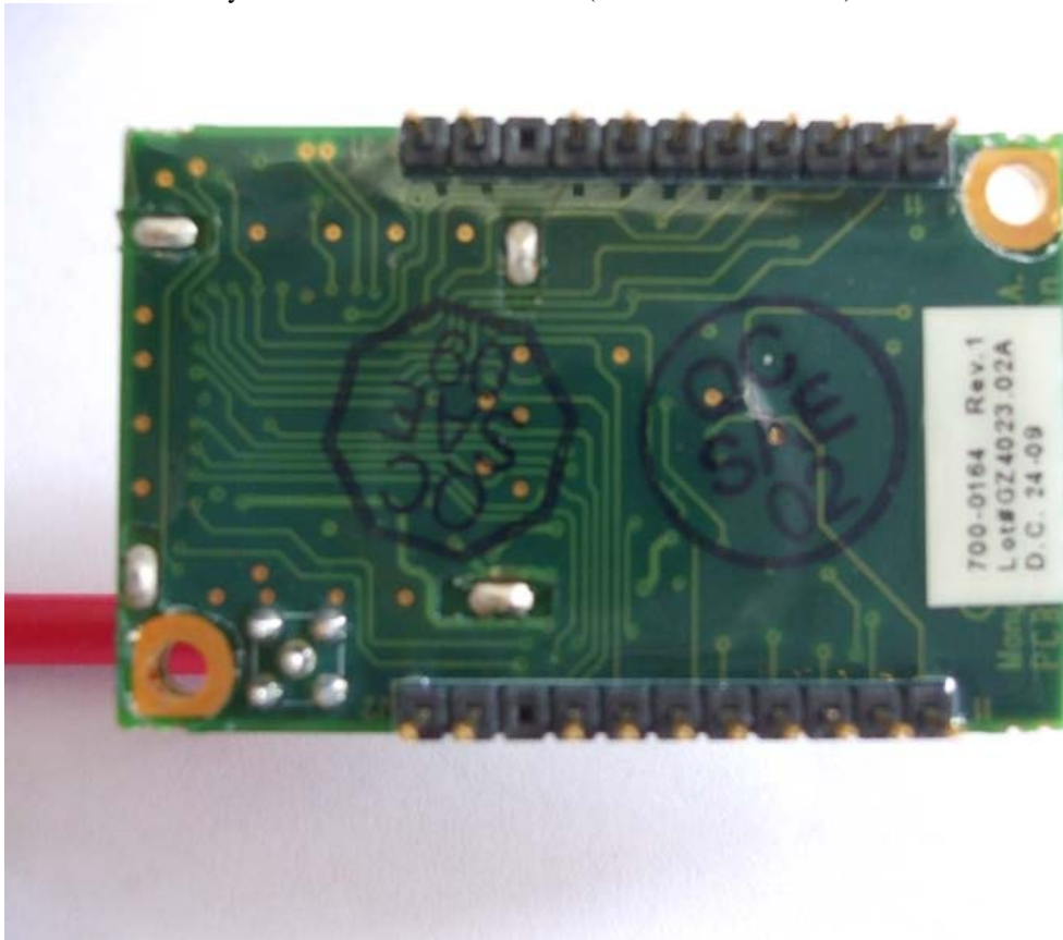
Rear of the ancillary Wi Hart radio module board (FCC ID: SJC-M2140).
