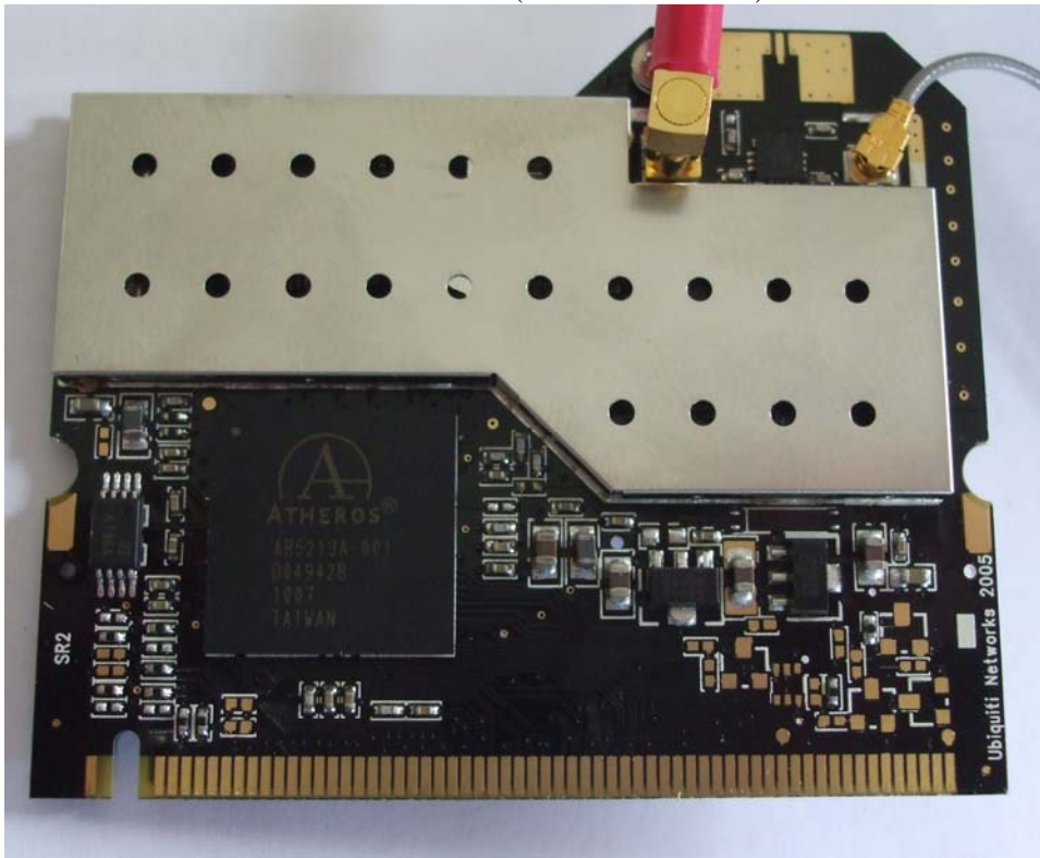
Rear view of the Wi Fi radio module board (FCC ID: SWX-SR2)
