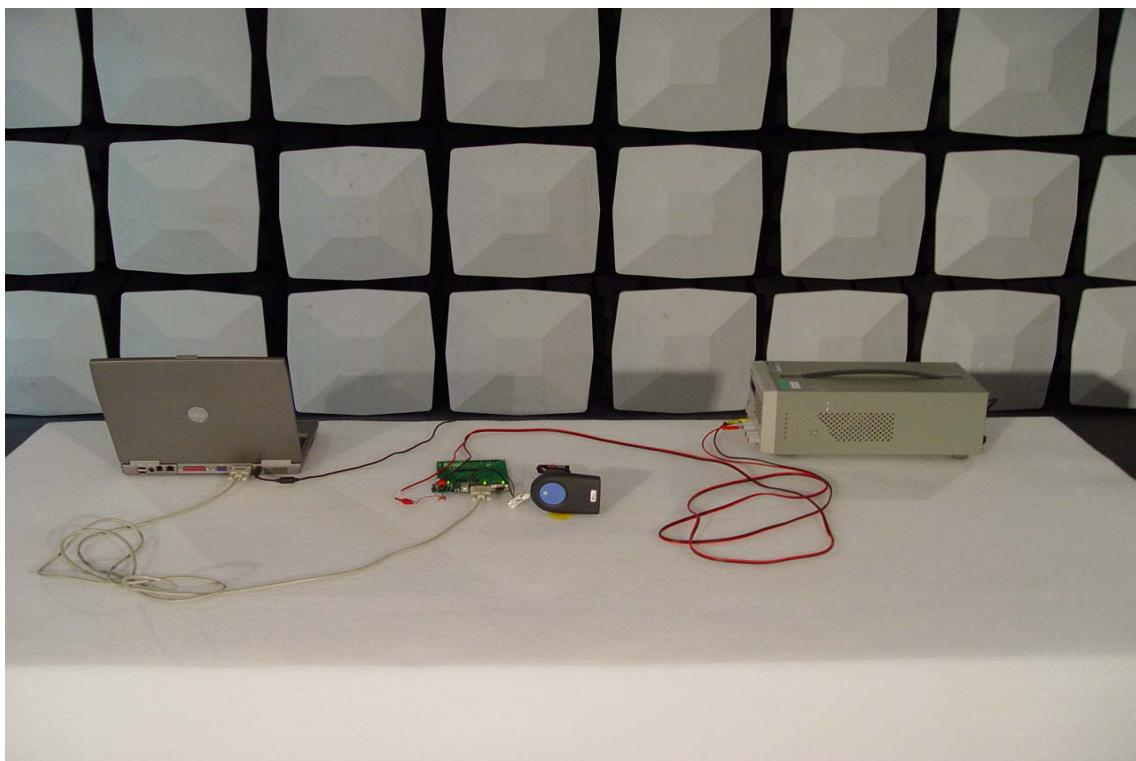
**Powerline Conducted Emissions Setup Photos**
