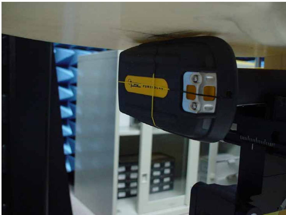
Fig.8 Photo of the EUT Right-on contact to the Flat phantom, Spacing between EUT and phantom –In contact (0mm)
