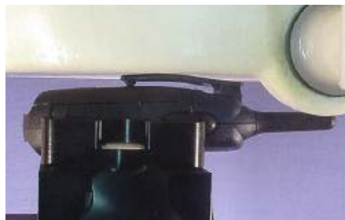
Body-worn SAR Test Setup 0.7cm Belt-Clip Separation
