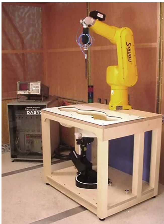
DASY3 SAR Measurement System with SAM Phantom
