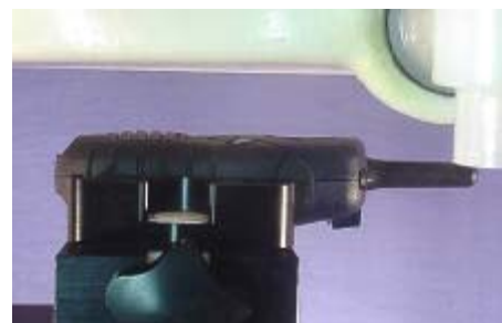
Face-Held SAR Test Setup 2.5cm Separation Distance
